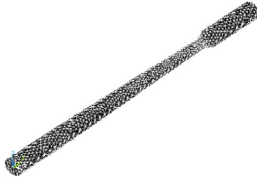
Fig. 10. Finite element model of aluminum specimen.
